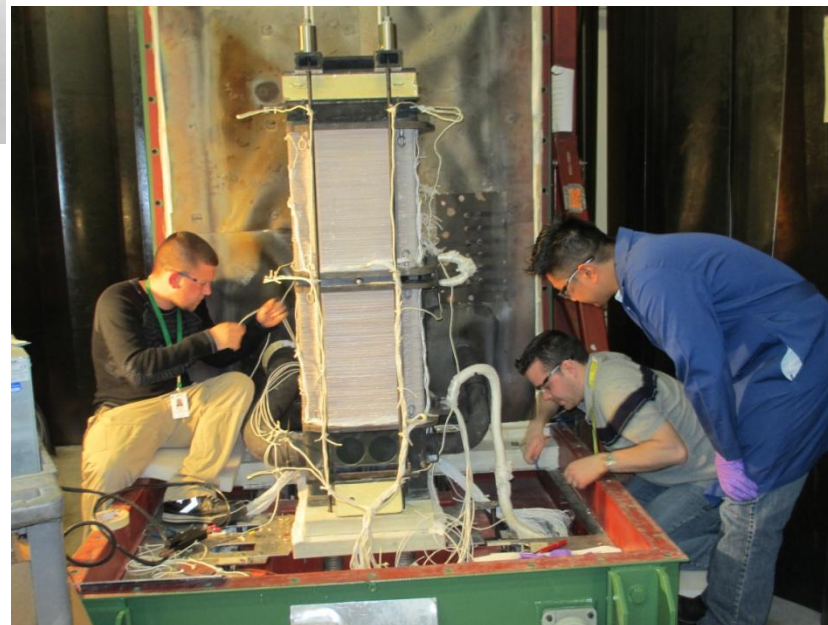
FCE/VPS SOFC 30 kW Stack Tower (192 cells) (2012)
